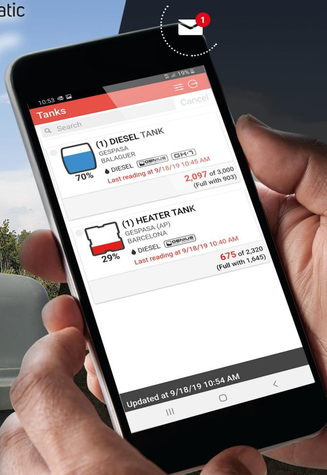
With the Dolphin system it is possible to measure the fluid of your tank and automatically send the reading to the web site [www.dieselplus.net](http://www.dieselplus.net) or your smartphone with the "DieselPlus Tanks" App.
